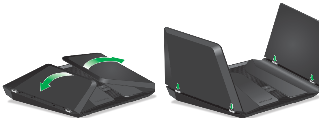
Figure 4. Position the antennas
