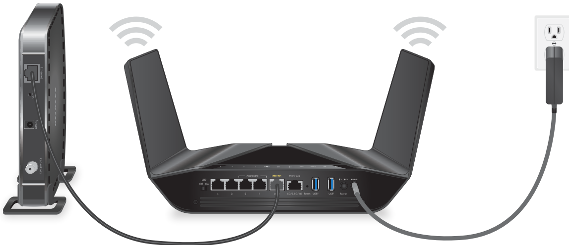
Figure 6. Cable your router
