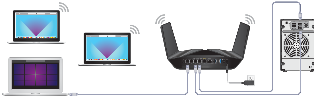
Figure 7. Ethernet port aggregation
